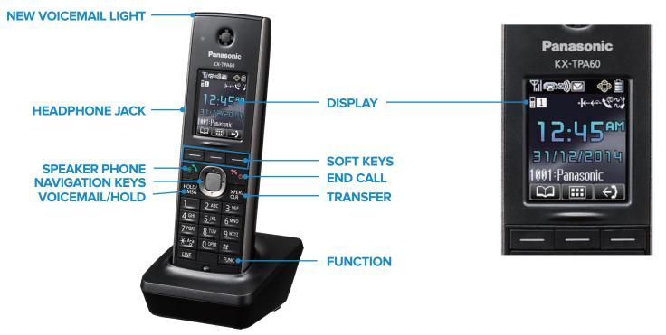
Below are display icons and soft keys that will appear on your phone screen. Display icons are indicators for items like signal strength and battery level. Soft keys are the three buttons located beneath the phone's display screen that allow you to select options such as phone book.
